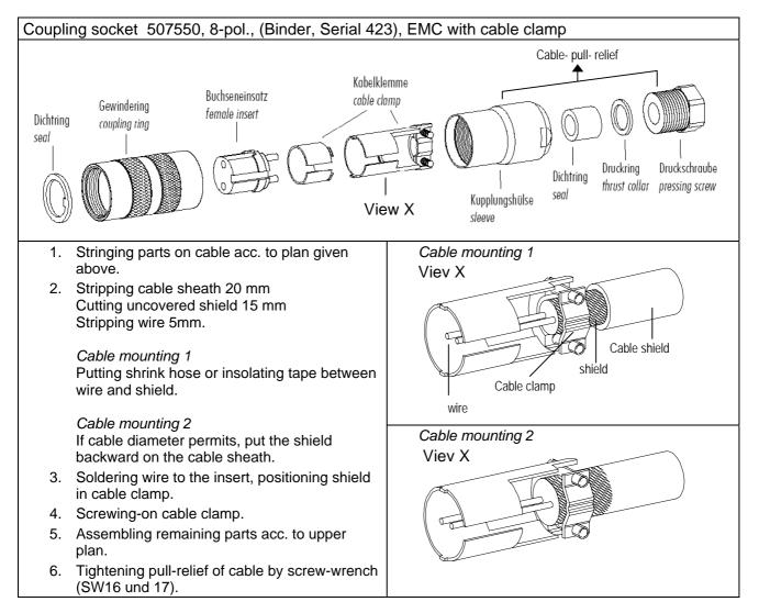
Fig. 1: Connector installation
